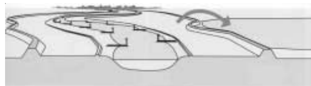
Figure 5. Schematic representation of detention polder for temporary or emergency storage of river water in the hinterland
