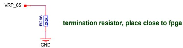
termination resistor, place close to fpga
