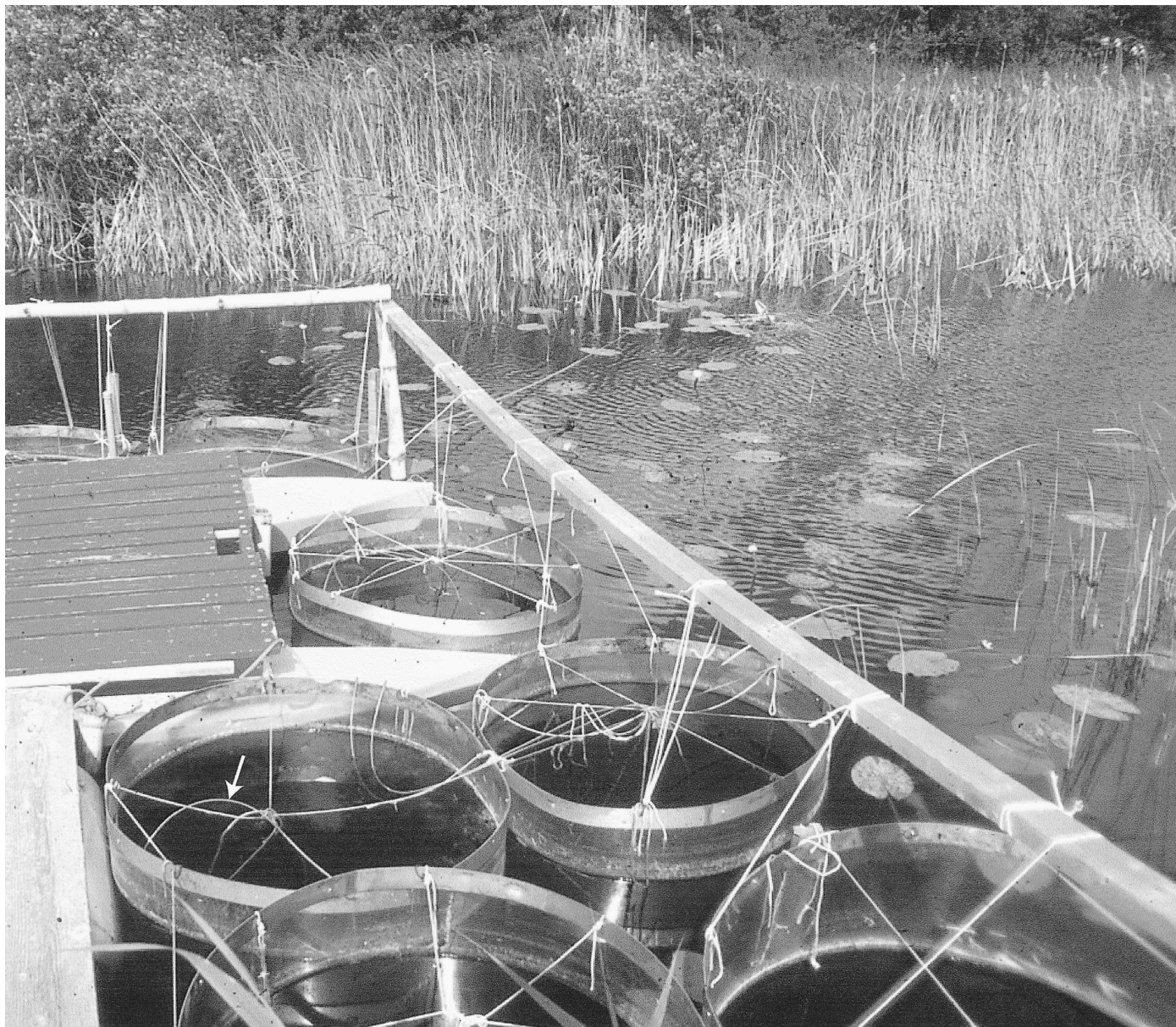
Fig. 1. Part of the experimental setup at the Weerribben location. Arrow indicates tubing connected to ceramic moisture samplers in the sediment.
