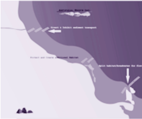
Figure 2a The mouth of La Antigua river with sediment diverted by wave attenuation devices. Further down the coast the natural reef and the Veracruz port are located. Source: Artificial Reefs, Inc., Florida.
