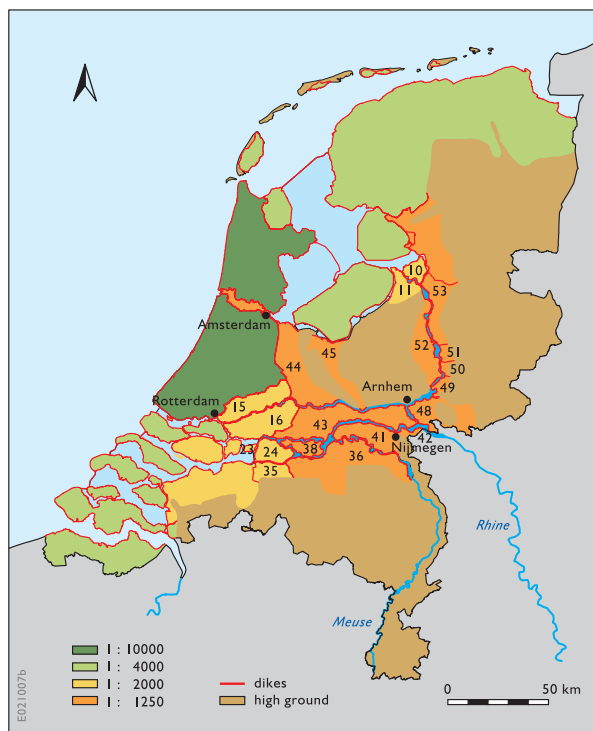
Figure 3. Dike-rings (numbered, referring to Tables 1 and 2) and safety levels along the lower Rhine River in The Netherlands.
