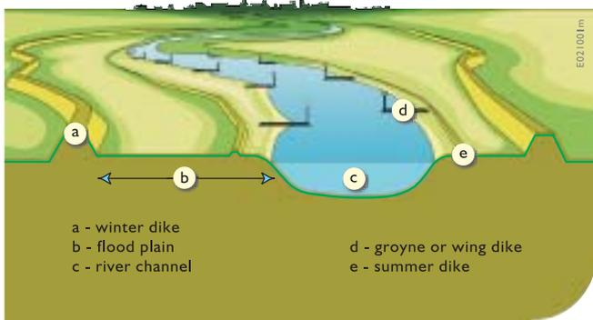
Figure 3 Two-tier dike structures and groynes for flood protection along the rivers in The Netherlands.
